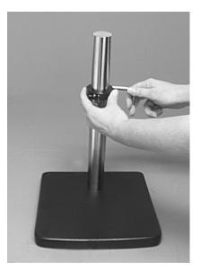
5. Slide the cross block onto the vertical post.
