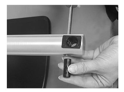
2. Unscrew the e-arm/focus mount locking screw and set aside.
