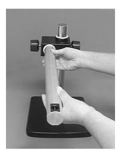
8. Set to desired position and tighten the cross block and horizontal pillar on both sides using the 2 knobs.
