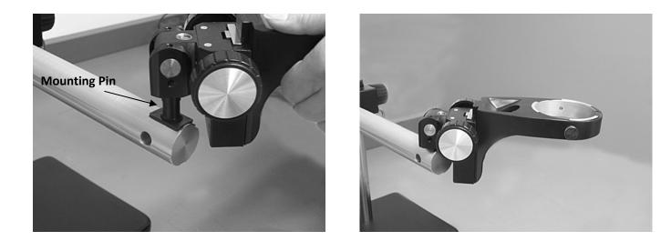
4. Adjust the e-arm or focus mount to desired position and then re-insert and tighten the e-arm/focus mount locking screw with the V grooves facing towards the mounting pin of the arm.
